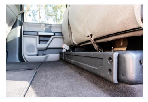
2. Starting on Driver Side. 4. Put (1) bolt through the middle hole in the seat bracket. Add (1) nut to hold in place. 4. Add second nut to bolt and then the washer. 5. Repeat on the next seat bracket in the middle
